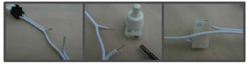
Cut one of the wires and bare its ends. Loosen the screw terminals of the switch. Insert each of the bared ends into one of the two terminals. Re-tighten the screws.
