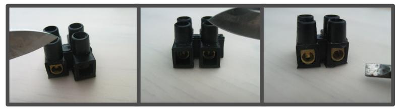
Use the knife to cut away all the plastic covering from one end of the connector block. The brass fittings should be exposed as above.
