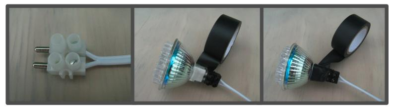
Begin to wrap insulation tape around the 'neck' of the spotlight. Go round a couple of times...
