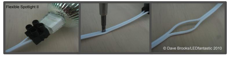
Insert the wires into the 'back' two terminals and close up the screws. Make sure they are tight. You can have the switch anywhere along the wire you like, but here I have chosen it to be near the bulb. Use the screwdriver to gently prise apart the two wires.
