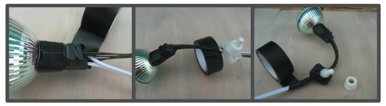
Continue wrapping the tape at an angle, down the wires until you reach the switch. Unscrew the switch collar before wrapping then put it back afterwards. You may need to have a few goes at wrapping the switch and you could even tape it up first to make a neater job. You have plenty of tape. Its ok to cut the tape too – this doesn't have to all be done in one long run. Wrap down to the end of the modelling wires.
