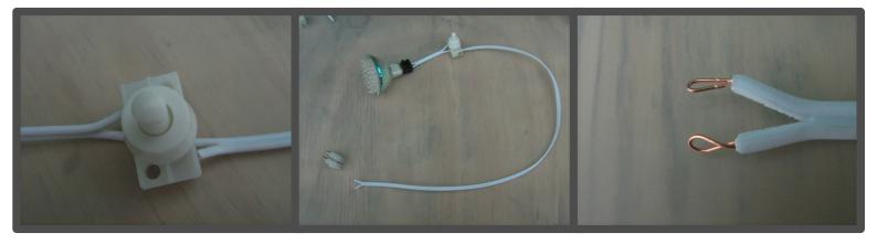
Bare the other ends of the wire and insert them in the male half of the connector socket. The female side should be connected to your 12v power source.
