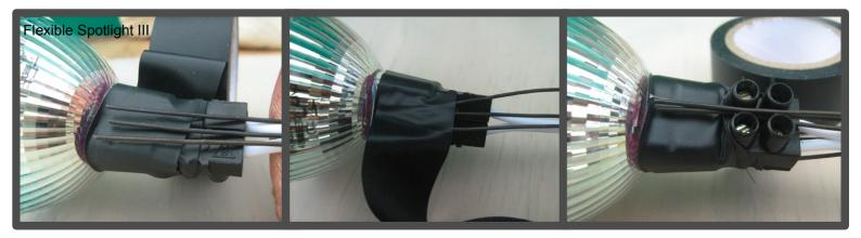
Lay half the modelling wires 'on top' of the taped connector and bulb-neck. Tape firmly in place – go round a few times. Lay the rest of the modelling wires 'underneath' and continue wrapping tape around the neck of the bulb until all is firm.
