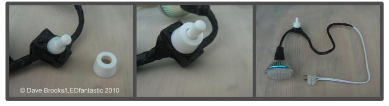
Tape the end of the modelling wires (where the tape wrapping finished) firmly to the spring clip. Attach the female connector to 12v & your job is done.
